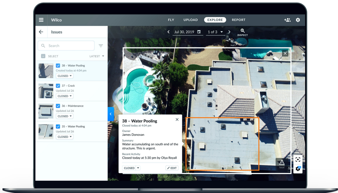
Figure 4. DroneDeploy can assist in monitoring and finding problem areas in a building.
